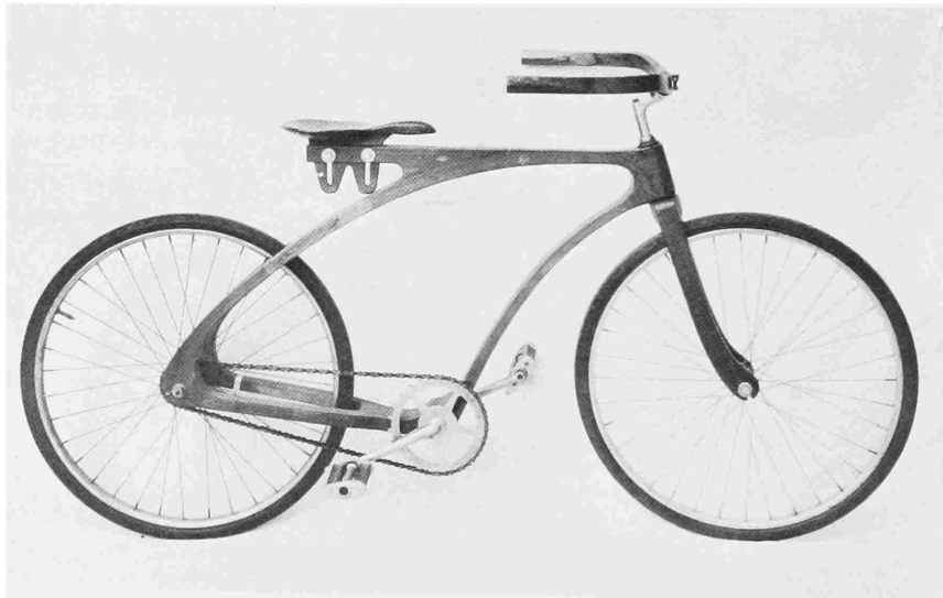
Experimental wood-frame Whalen & Janssen bicycle of 1942.
