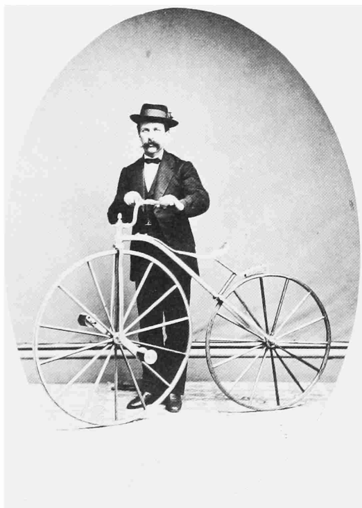
An 1869 Pickering velocipede in a rare contemporary photo that shows the rear saddle brace supported by a spring, so that a backward movement of the rider's body brings a brake-shoe down against the rear wheel.
