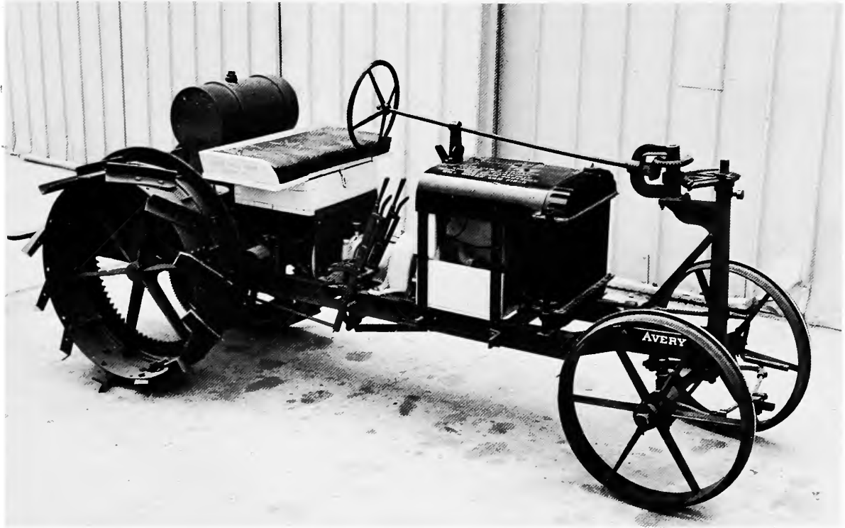
FIGURE 15.—Avery Bulldog tractor, about 1919. (Catalog No. 142.)
