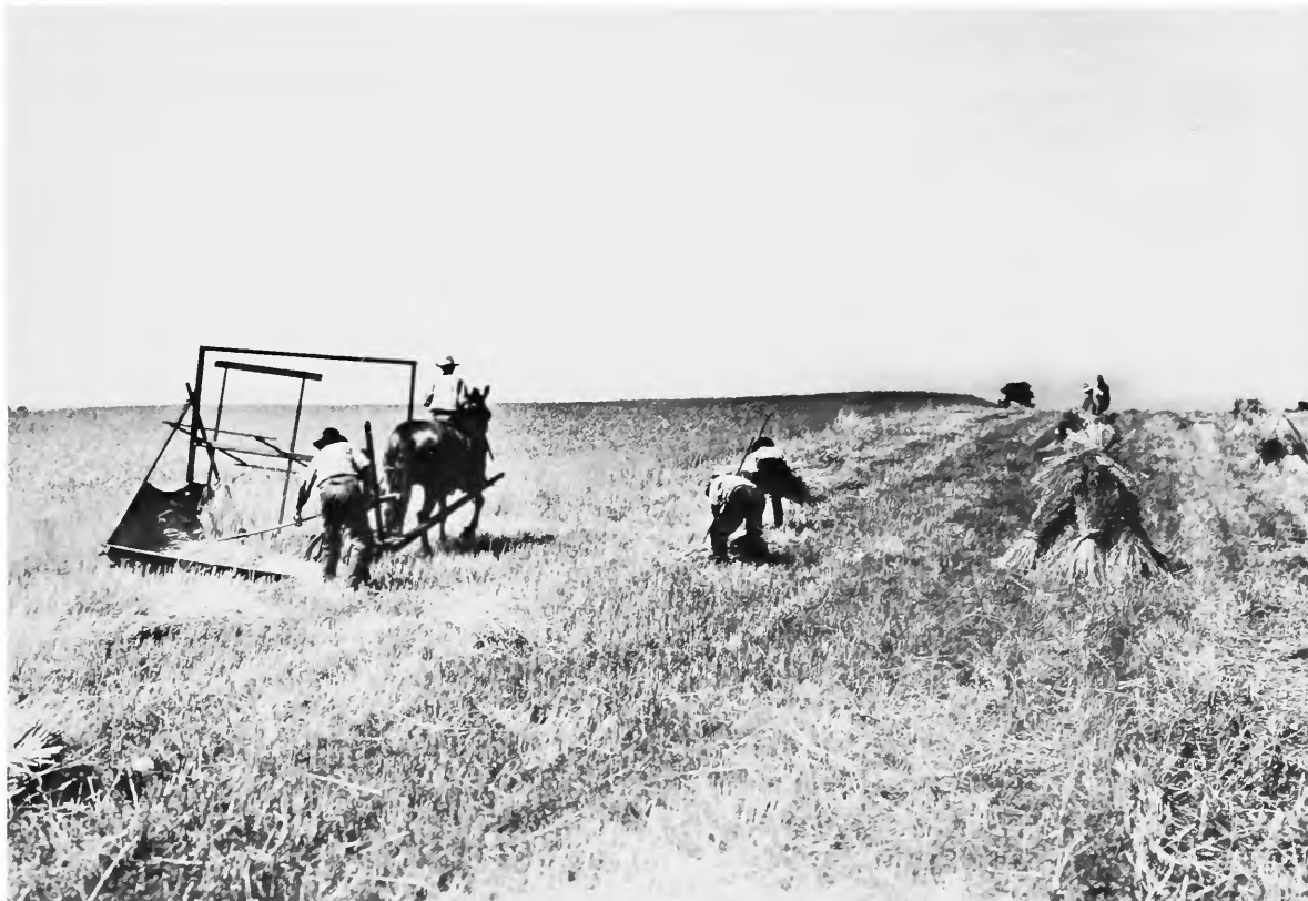
FIGURE 10.—McCormick reaper (1831) in use in the field. Photo courtesy of International Harvester Corporation. (Catalog No. 98.)
