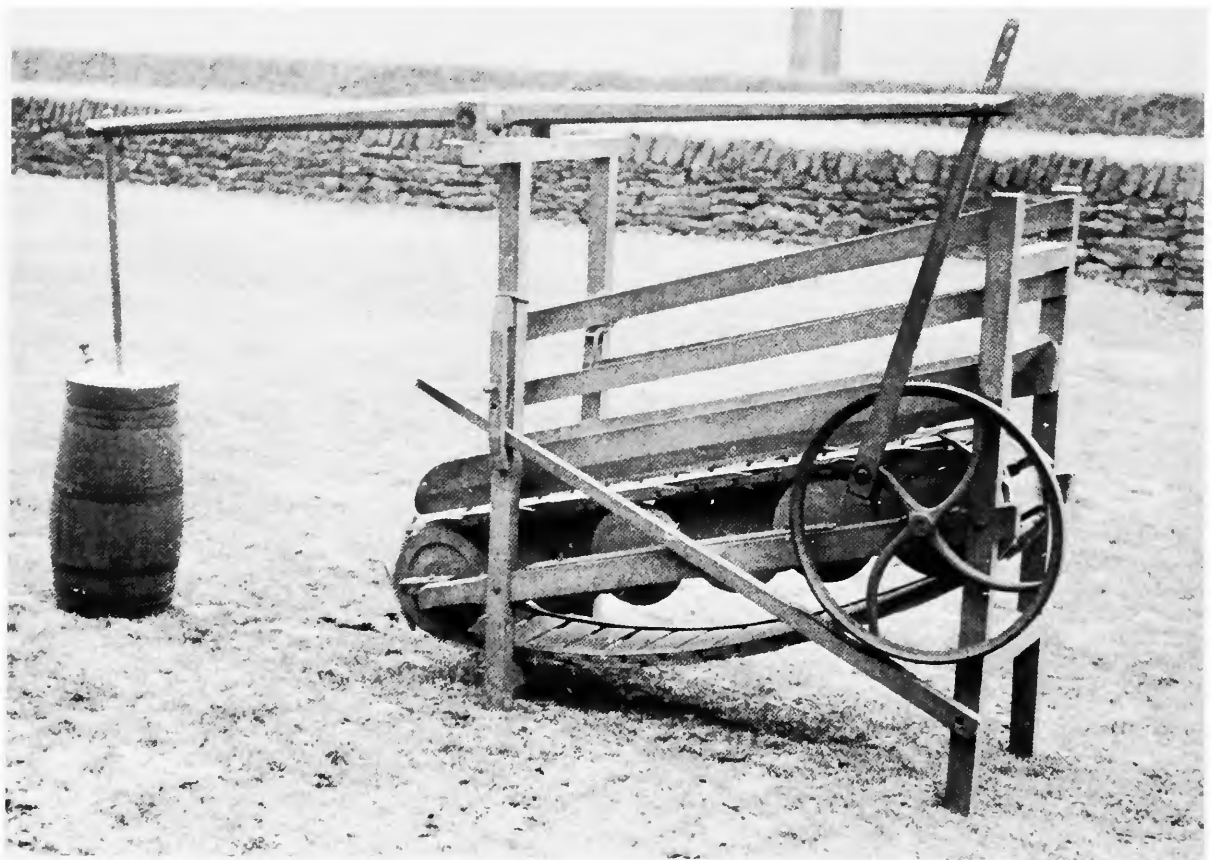
FIGURE 14.—Dog-powered churn, 1881. (Catalog No. 140.)
