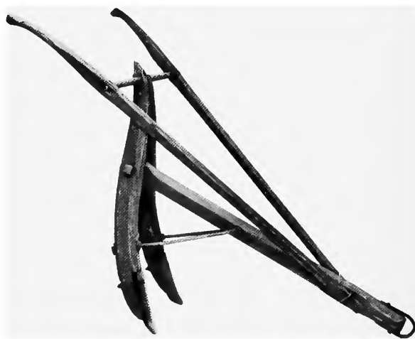
FIGURE 17.—Double-shovel plow. (Catalog No. 181.)
