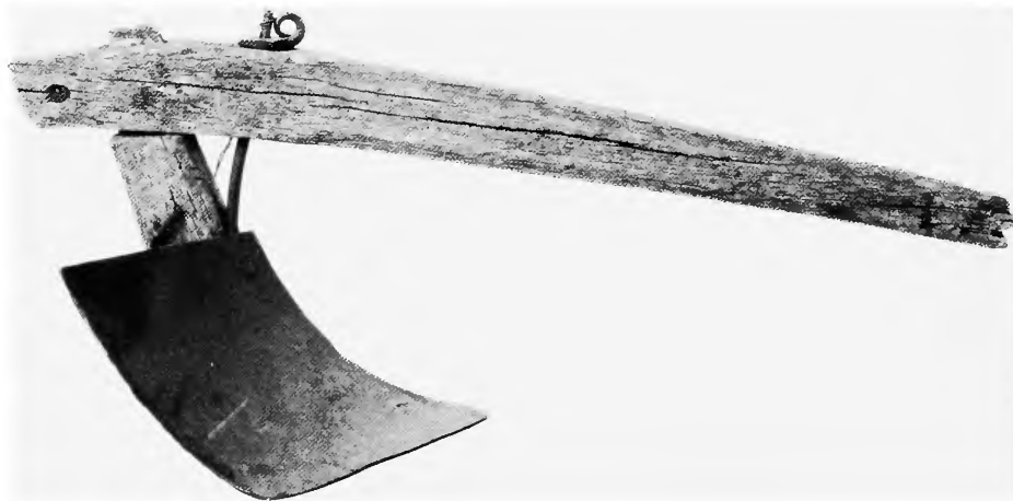
FIGURE 5.—John Deere plow, one of the three plows made by Deere in 1838. (Catalog No. 42.)
