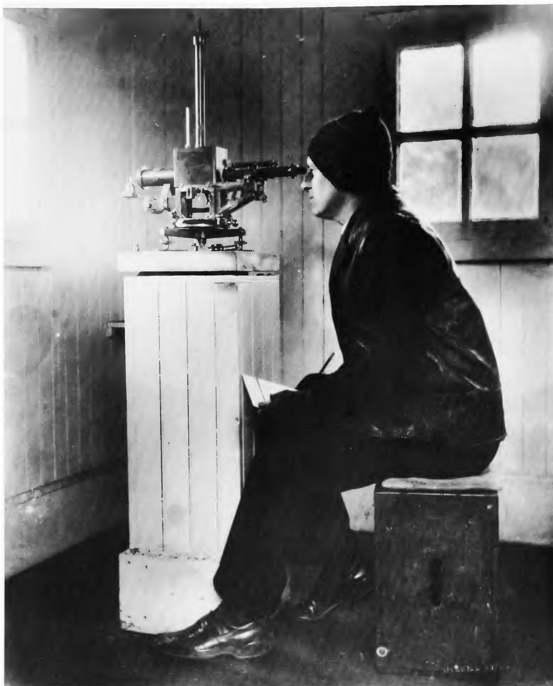
FIGURE 50.—No. 21 (?), Magnetometer, British India Survey Pattern.
