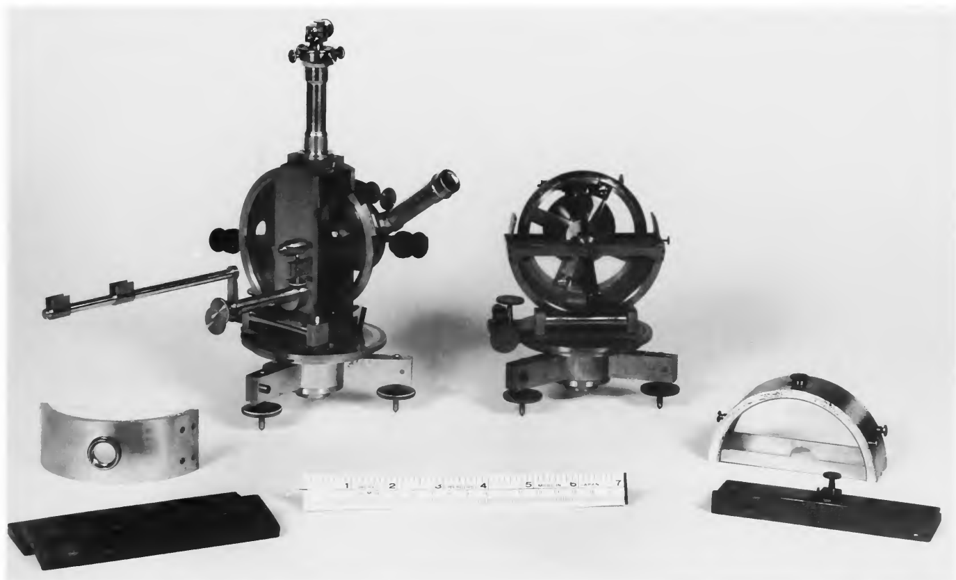
FIGURE 64.—Nos. 10 and 35, Magnetometer (left) and Dip Circle (right), Brunner-Chasselton, ca. 1884.
