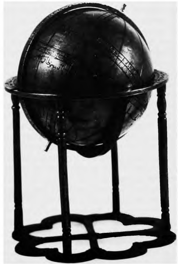
FIGURE 34.—Globe No. 113, unsigned and undated. This globe has no stars and the unusual feature of a graduated solstitial colure. Paris, private collection. (Photo: Alain Brioux)
