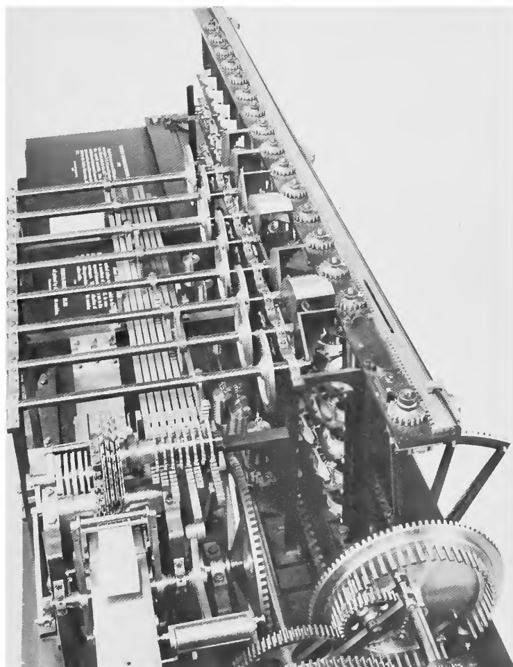
FIGURE 11.—Top view of Scheutz calculator showing printing apparatus. (SI photo 74-11261)
