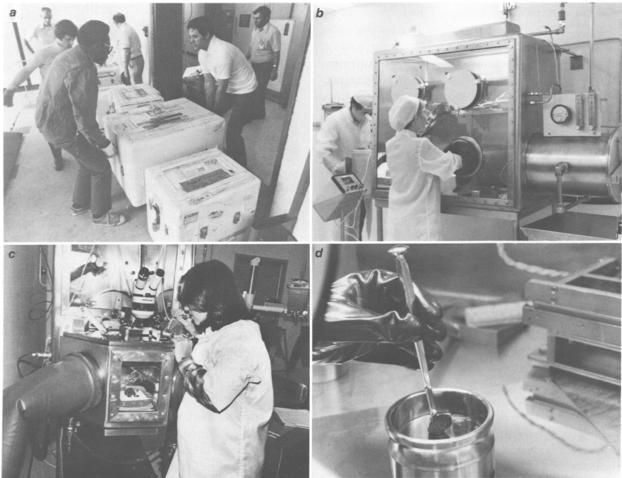
FIGURE 6.—Processing Antarctic meteorites at Johnson Space Center, Houston: a , Arrival of the metal boxes containing the meteorites packed in dry ice. b , Inside the stainless steel, controlled-environment cabinets with a nitrogen atmosphere, the meteorites are weighed, photographed, dried, and chipped. c , Observation port of a processing cabinet, through which a meteorite is visible on the photo stage. d , Meteorite being chipped inside the processing cabinet; the chisel and bowl are of stainless steel.
