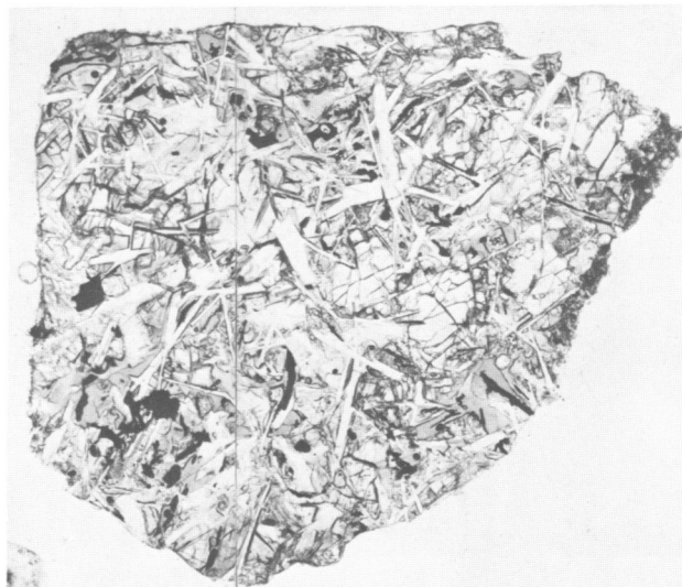
FIGURE 1.—Thin section of basalt fragment from Apollo 15 soil sample 15272,11. Maximum dimension of fragment 2.0 mm. Transmitted light.
