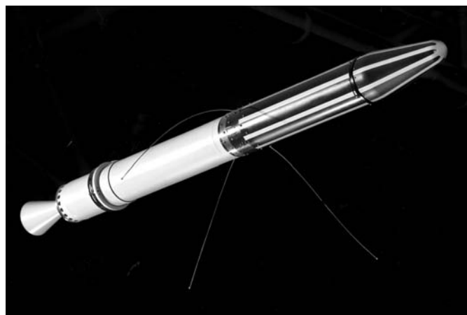
FIGURE 6. Explorer 1 (A19620034000), initially displayed in the Smithsonian’s Arts & Industries building, became a centerpiece in NASM’s Milestones gallery upon opening in 1976. Opening it for inspection revealed it was a true backup but was devoid of instrumentation. (NASM photograph)
