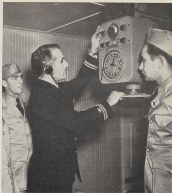
Officer candidates (deck) learning use of the radio direction finder for a bearing
