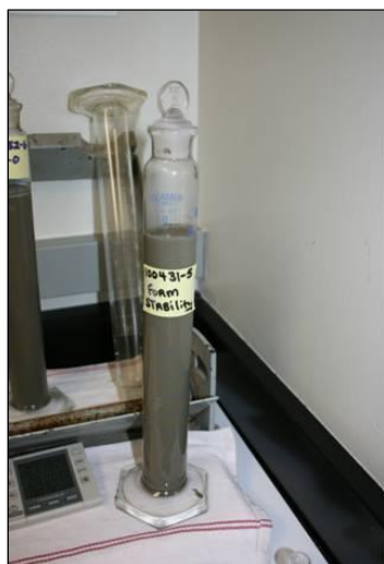
Figures 4.4.2 and 4.4.3. Foam testing apparatus.
