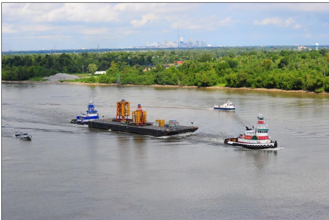
Figure 4.9.1. Transporting the Deepwater Horizon BOP.
