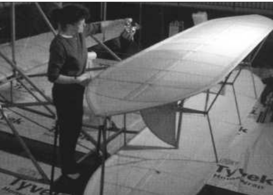
A technician restores the fabric-covered wing of the Wright Flyer.
