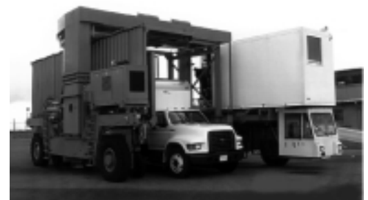
Figure 7. Mobile Container X-Ray System
