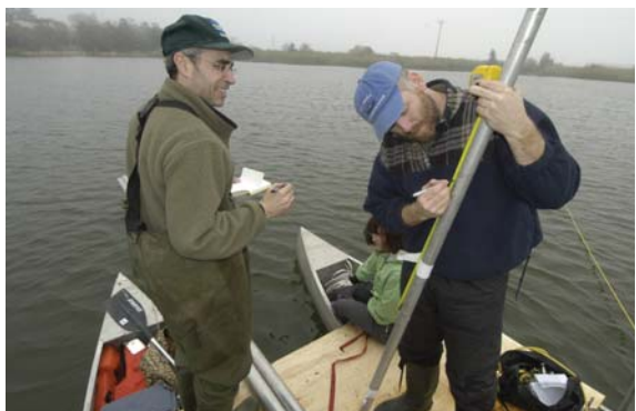
Jeffrey Donnelly (right) of the Woods Hole Oceanographic Institution (WHOI), and his colleague, prepare to extract a sediment core from Oyster Pond, Massachusetts. Donnelly is studying climate change by looking for evidence of major hurricanes over centuries recorded in the sediments of coastal areas. Credit: Tom Kleindinst, Woods Hole Oceanographic Institution
