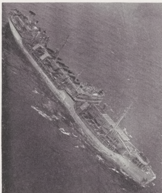
Special decks were laid on tankers to carry war planes and other dry cargo.
