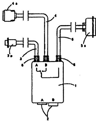
The device described in Yamada also has a set of connector ports (A & B) that are electrically coupled to the switching circuit. In addition, it has three cables (3, 4, and 5) that are “fitted into the main housing unit 1 directly with one end of the cable via a protective ring 6.” RX-522 at 2(0009). Figure 2 more clearly shows the protective ring 6 and shows that it has a lip on the inside and outside of the housing so that the attachment element connects the cable fixedly to the housing and
