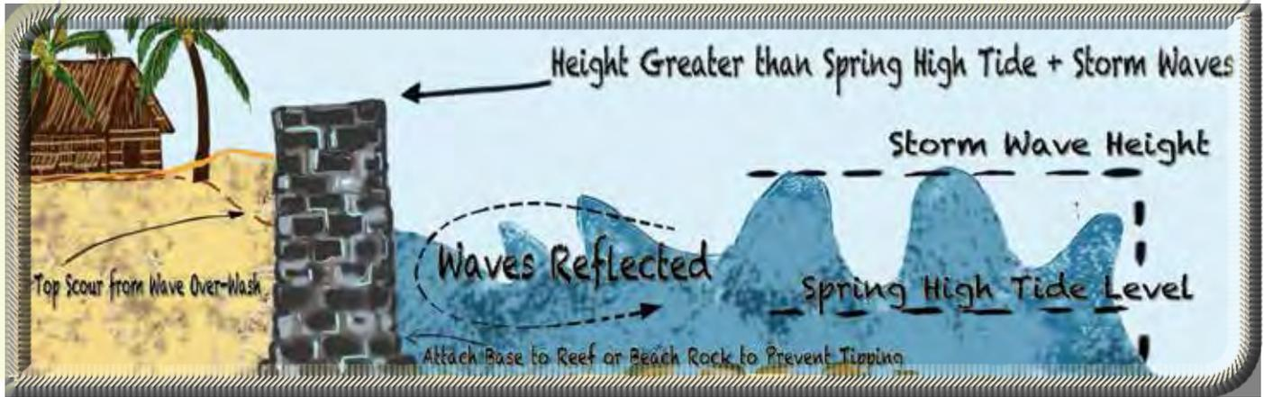
Seawalls act to block waves and water motion from interacting with land. Seawalls reflect wave energy away from the shore.
