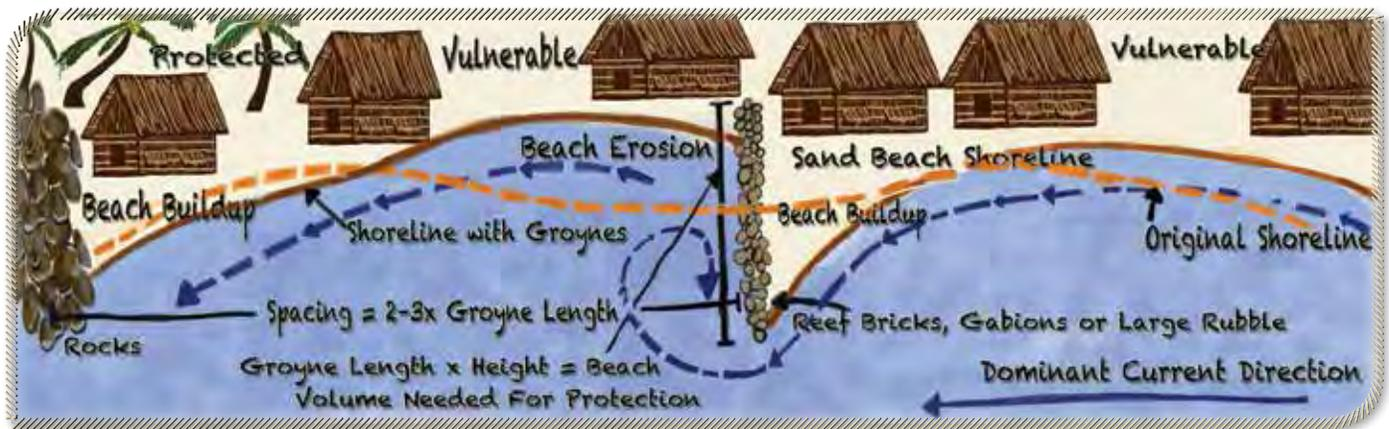
Groynes trap sediment from traveling along the shore. Trapped sediment accumulates to increase beach area that is up-drift of the structure. This is often balanced by erosion leeward of the groyne and at down-drift shores.
