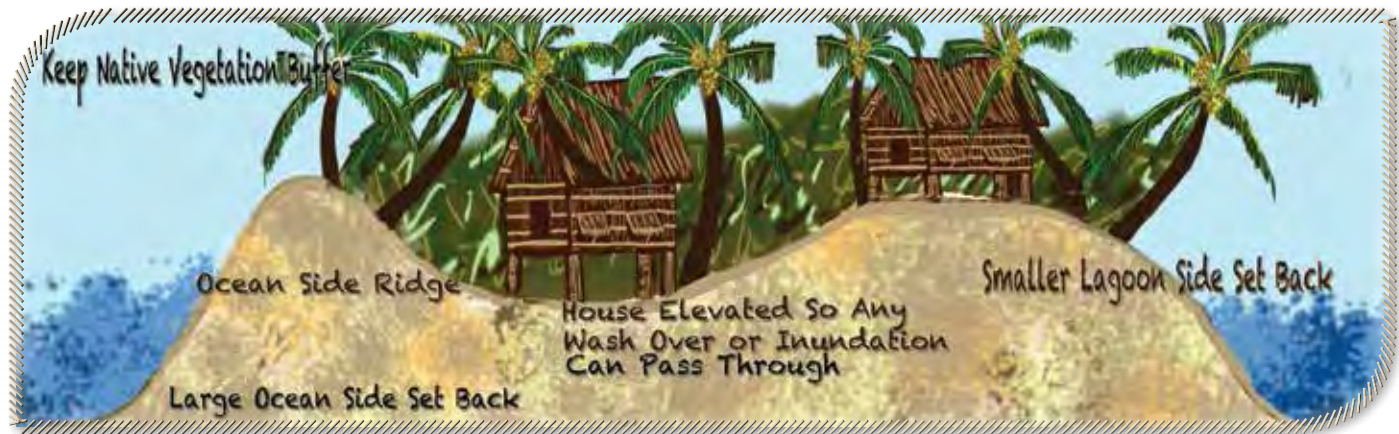
Profile view of an island with lagoonal and oceanside setback zones and raised floor levels; these measures allow for natural island movement.
