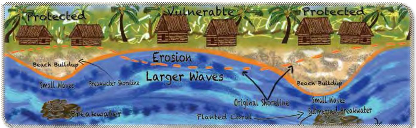
Breakwaters work to protect the shore in two ways: 1) By dissipating wave energy offshore, before waves reach the shore. 2) By changing nearshore processes, breakwaters cause sand to build up behind them (only if there is a sandy shoreline).
