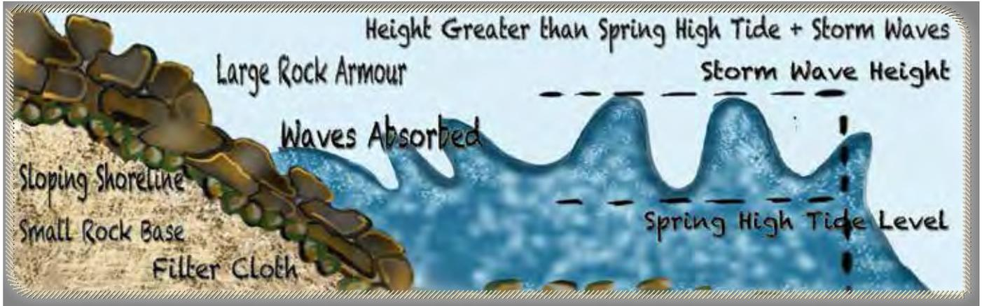
Revetments stop wave energy from interacting with land by absorbing and reflecting wave energy away from the shore. Depending on material and construction, revetments may not be high enough to block extreme water levels.
