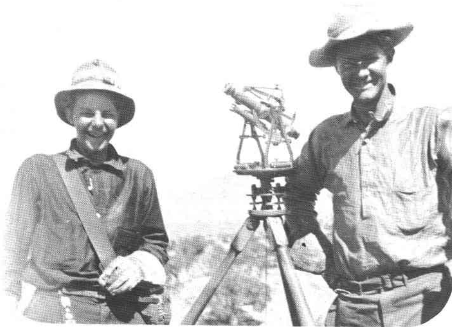
Hopi Indian Reservation, Arizona, 1910. Left to right: Ty and Van White. The instrument is a Gurley with a Burt solar attachment.
