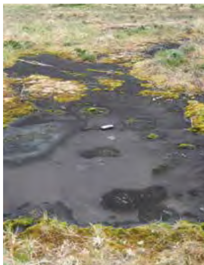
Pyramid Cove barrel and burn pit area with POL saturated soil on Attu. D. Rudis, USFWS
