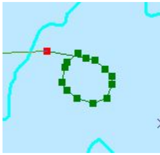
Figure 29 – Step one of the isolated polygon addition process.
