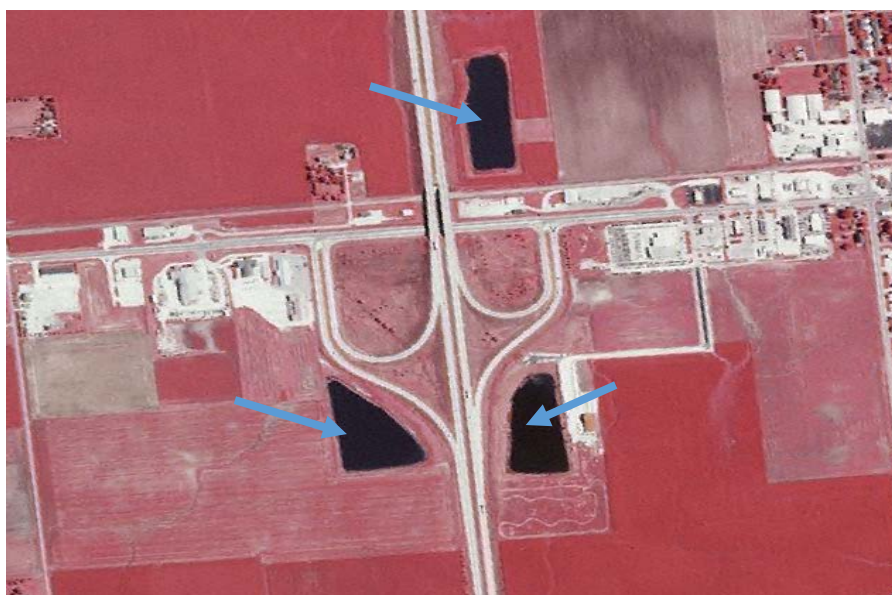
Figure 16 - Borrow pits (indicated by the blue arrows) found in association with a highway interchange. The shape and proximity of these ponds to the highway interchange provide good indicators for descriptive categorization.
