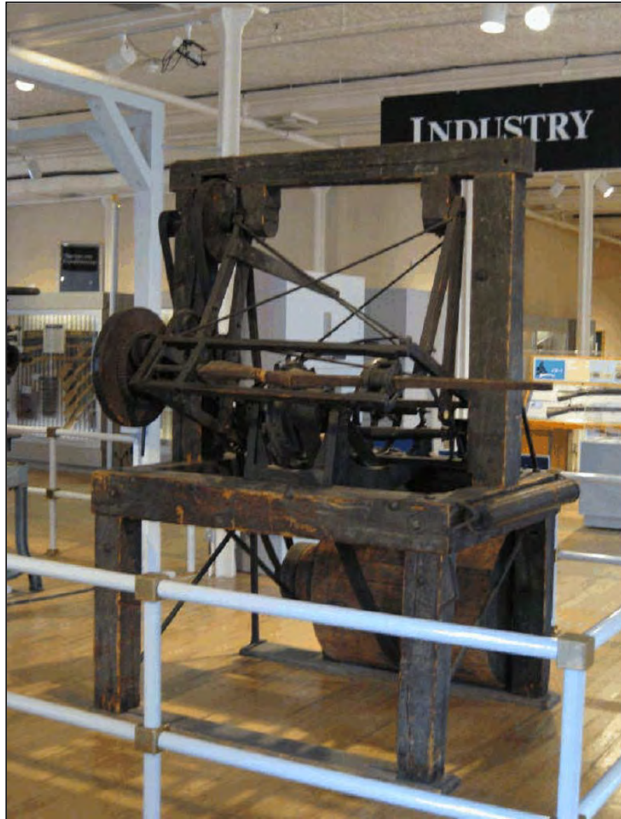
Figure 4.3. Another of the Main Arsenal's most important exhibits: the Blanchard lathe (photo: author).
