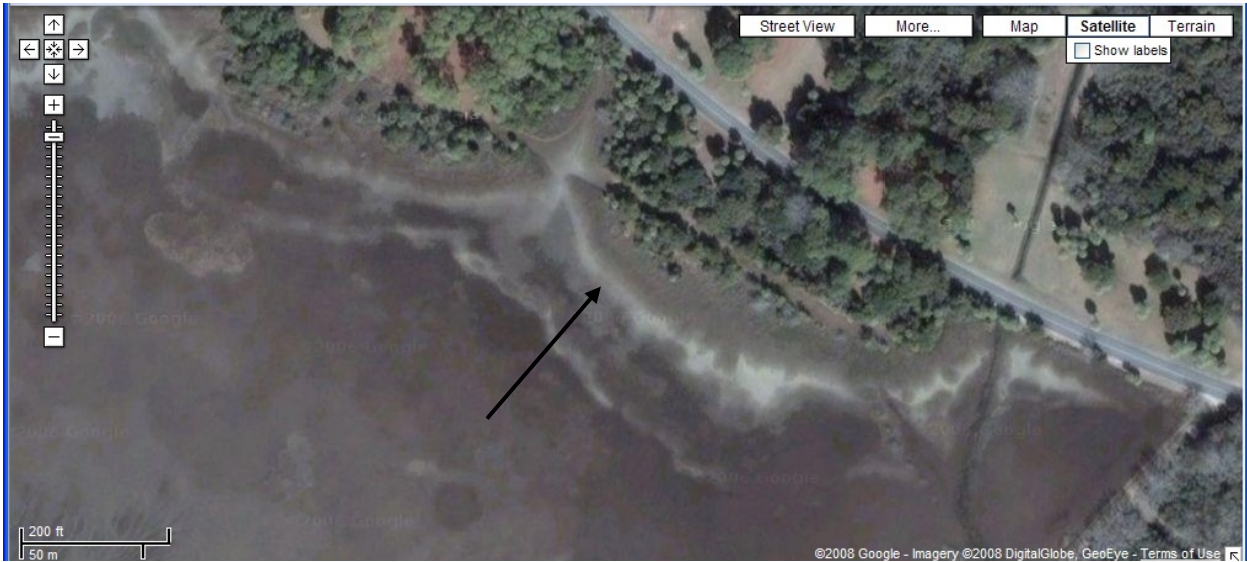
Figure 53. White areas on fringes of nontidal dredged spoil deposits and uplands next to tidal marshes may indicate poor vegetation from low pH or high salinity, or poorly-vegetated sandy sediment washed free during extreme high tides (Google 2008).
