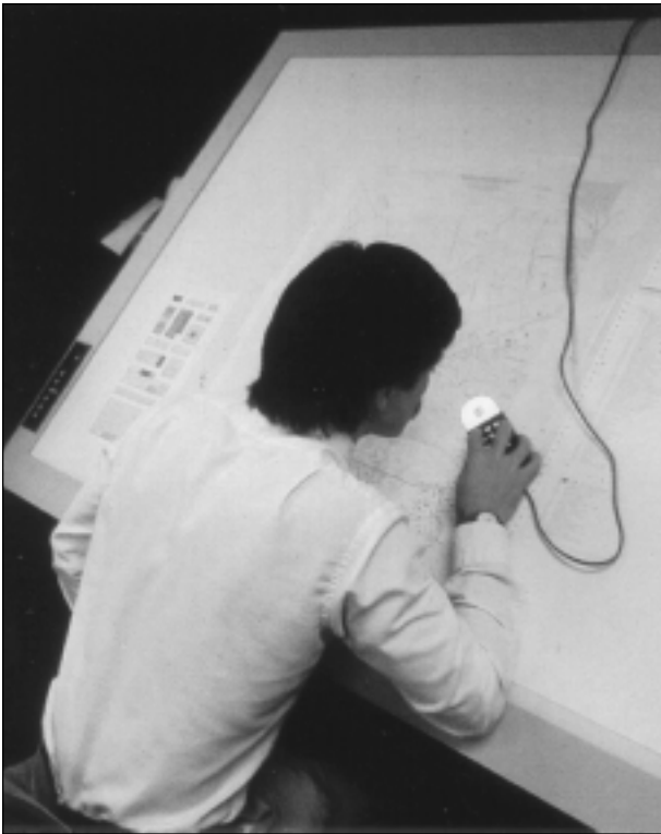
Figure 4. Digitizing converts map information to digital form using a hand-held mouse. (USGS, 1995)
