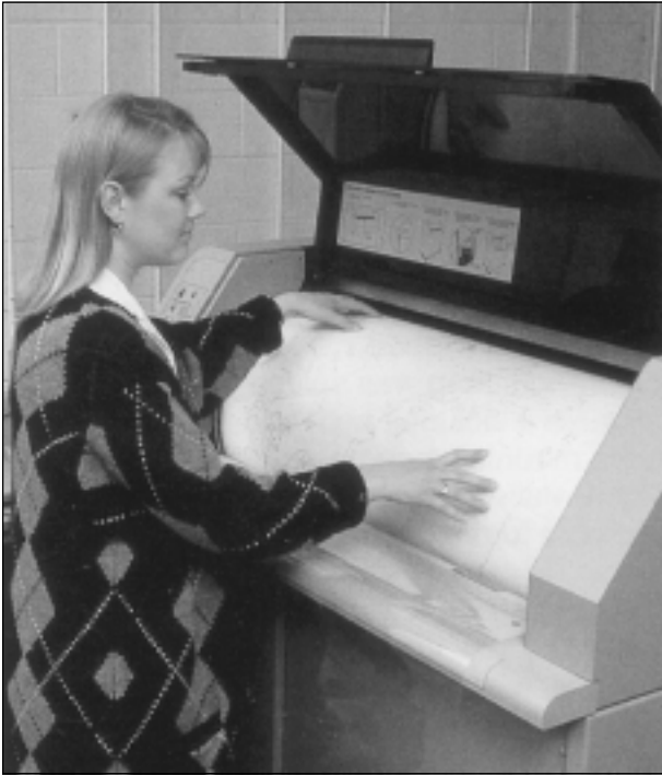
Figure 3. A large scanning device converts map information to digital form. (USGS, 1995)
