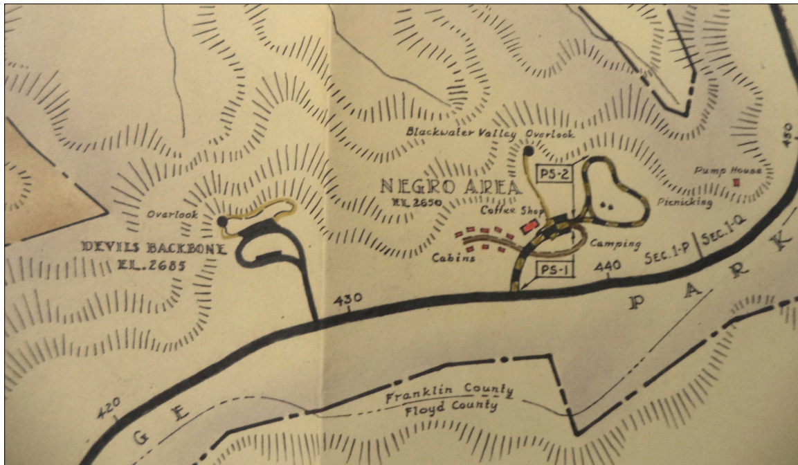
Figure 41. Details of completed and proposed development at Pine Spur from the 1945 master plan. The roadways marked as “under construction” had been treated with crushed stone, but were not hard surfaced. (Drawing PKY-BR-PS-2004, Drawer 1, Map Cabinet 2, BLRI Archive, Asheville, NC.)
