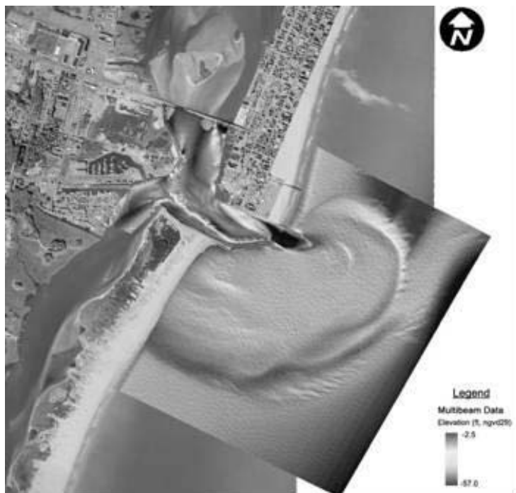
Figure 21. Comprehensive multibeam survey of Ocean City Inlet and ebb shoal, August 2005 (Buttolph et al. 2006).
