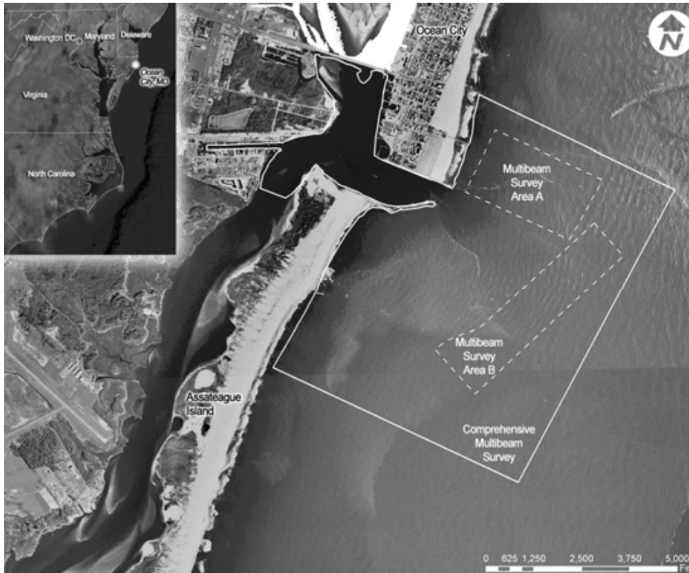
Figure 20. Boundaries of multi-beam surveys performed since 2003 from Buttolph et al. (2006).
