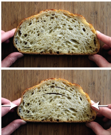
Figure 31. Formation of exfoliation joints, as illustrated by Glazner and Stock (2010, p. 152) using a piece of sourdough bread. Two curved slits cut parallel to the convex upper surface (upper photograph) open when the bread is squeezed from the sides (lower photograph), illustrating how horizontal compression combined with a curved surface generates vertical tensile stress and, ultimately, exfoliation joints. Photographs courtesy Greg Stock (Yosemite NP).
