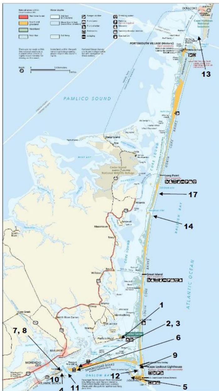
Figure 35. Location of coastal engineering structures impacting the park. Figure 13 from Coburn et al. (2010). Table 12 lists the erosion control structures and dredging locations (numbers indicate location in figure).
