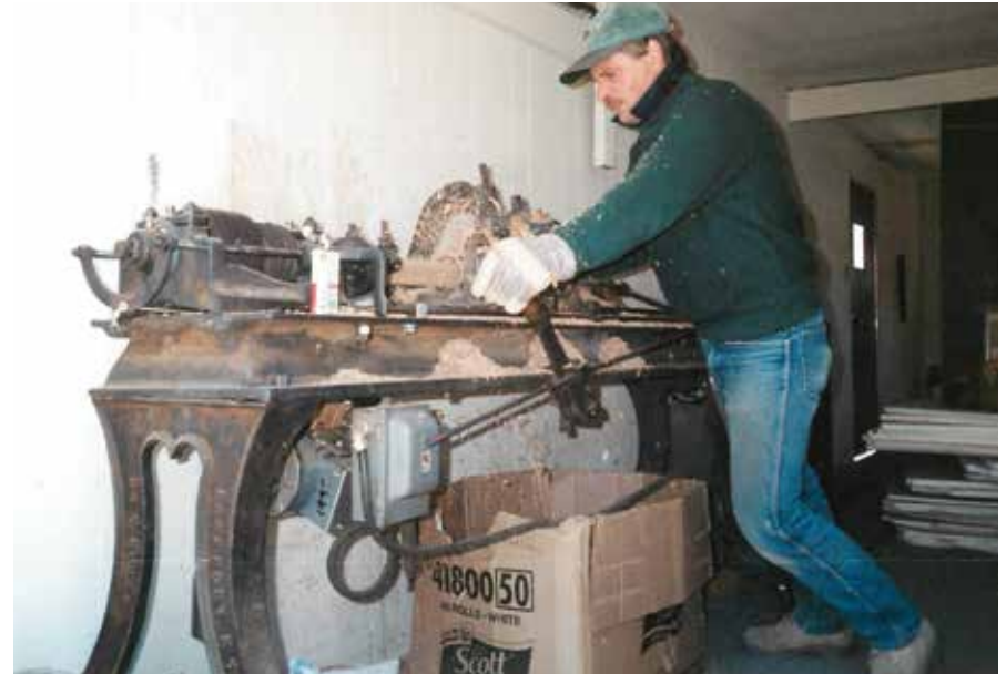
Figure C1.11 Tim Andrews fabricating replacement treenails on his Trevor treenail lathe. Sean T. James, 1998.
