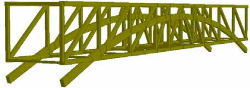
Figure C8.7 3-D Rendering (STAAD Model) of King's Bridge. SCLA.
