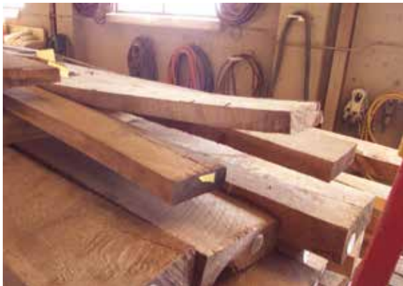
Figure 1.3a-b Seasoning timbers outdoors, even over a snowy winter, is the preferred method of drying structural timbers, time permitting. Below, white oak timbers being air-dried in a heated garage. While the drying process is expedited, the exterior of the timbers dry quicker than the interior, which can cause checking or warping. (Note that checks on compression members don't affect its structural capacity.)
