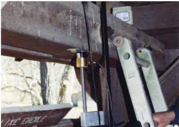
Figure 2.2a Copper naphthenate is an excellent preservative to protect from moisture infiltration, recommended to be painted on each timber to timber joint. Figure 2.2b Ultrasound field testing at the Salt Creek Covered Bridge, OH. The transducers read measurements which identified defective members in need of replacement.
