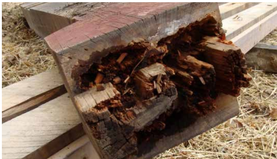
Figure C5.5 This photo of the top of a post shows the typical condition of truss members between joints. Timothy Andrews, 2009.
