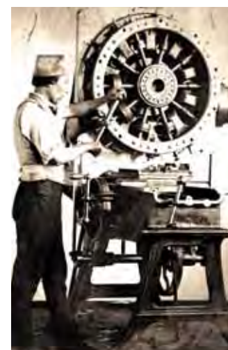
Right: At the time of the Civil War, the Colt factory used 450 mechanized steps in the process of manufacturing a revolver. This revolver frame jigging machine was designed and patented by Samuel Colt to cut the exterior and interior surfaces of a frame. Photo ca. 1857. Museum of Connecticut History.
