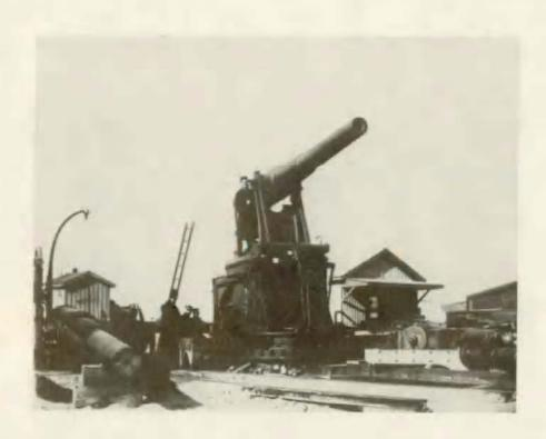
Photograph No. 16. Buffington-Crozier counter weight carriage by possible 10-inch rifle mounted for testing.
