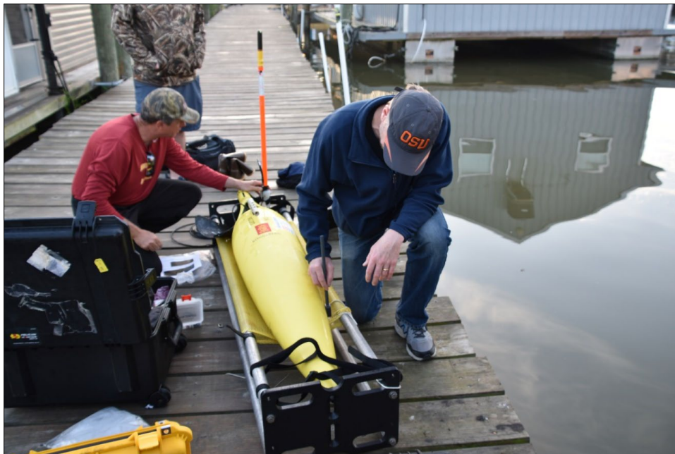
Photo C-17. Turning the Seaglider using a magnetic key.
