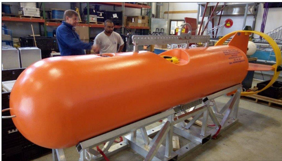
Photo C-12. StableMoor® buoy for the Canyon SHRU VLA.
