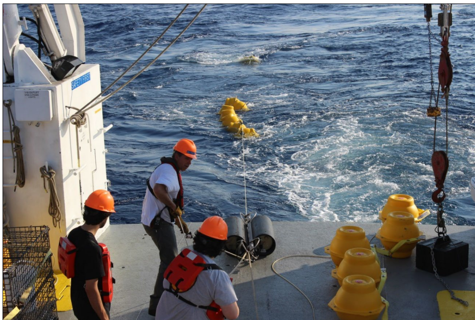
Photo C-6. EARS mooring deployment, top floats in the water.
