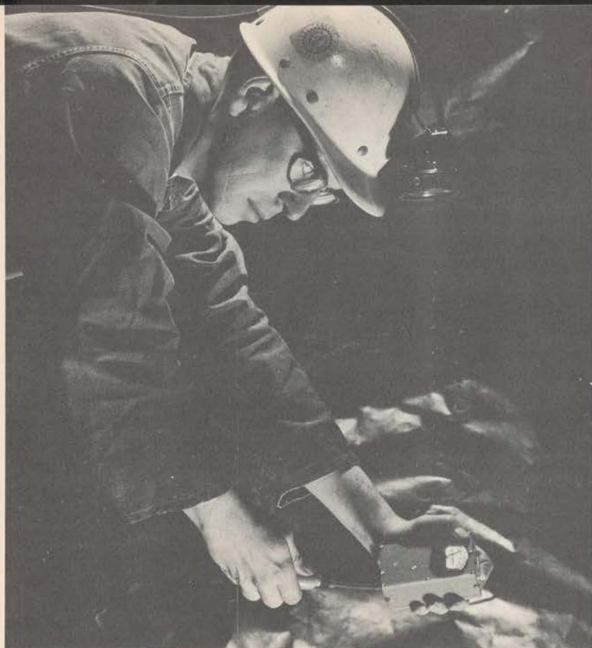
A new device for detecting combustible gases, developed by the Bureau of Mines, is demonstrated here in an underground mine.
