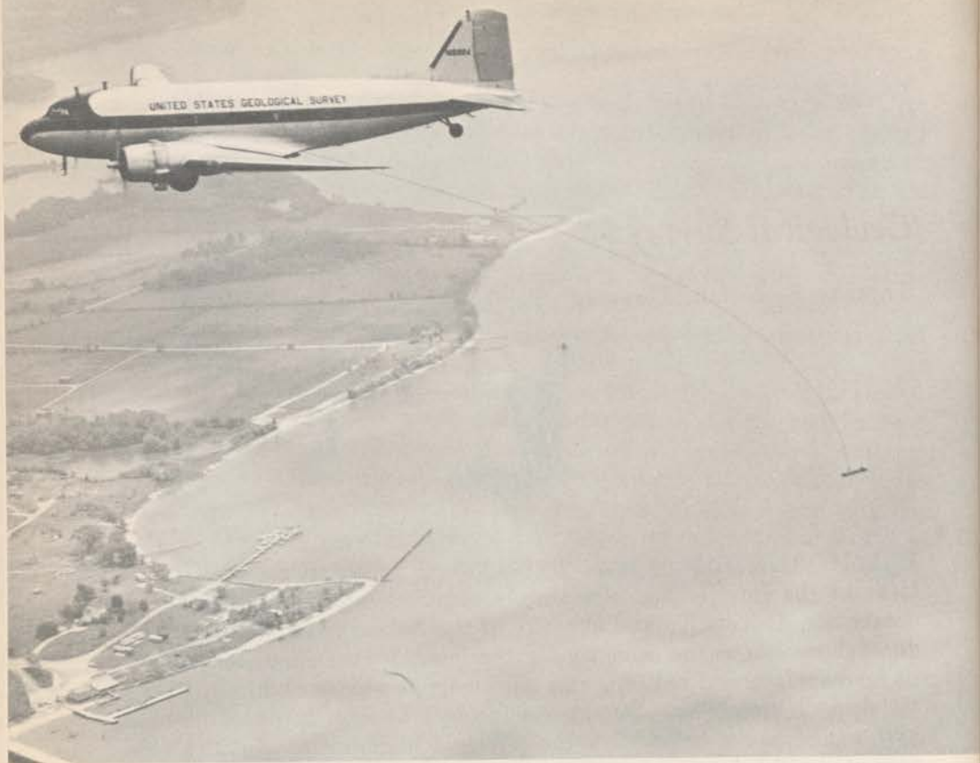
Measuring the earth's magnetic field, a Geological Survey aircraft with trailing magnetometer traverses Chesapeake Bay.
