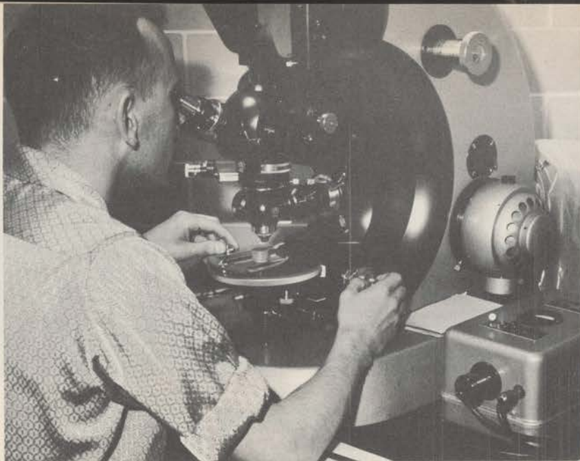
Mineralogists and petrologists use this ultraphoto microscope for examining mineral specimens at the Bureau of Mines' new research station, Fort Snelling, Minn.
