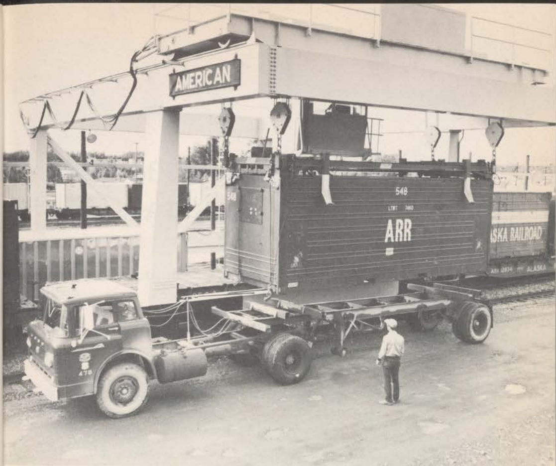
The Alaska Railroad's new Gantry crane, able to lift 40 tons, makes child's play of unloading one of the railroad's cargo containers from a flatcar to a waiting truck. The crane has greatly speeded the process of switching from train to motor truck.
