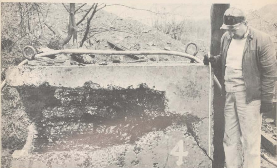
Tests in mining with powerful jets of water included those on anthracite. For this experiment, a block of anthracite was encased in concrete. Water jets cut deeply into the hard coal and even penetrated the surrounding concrete.
