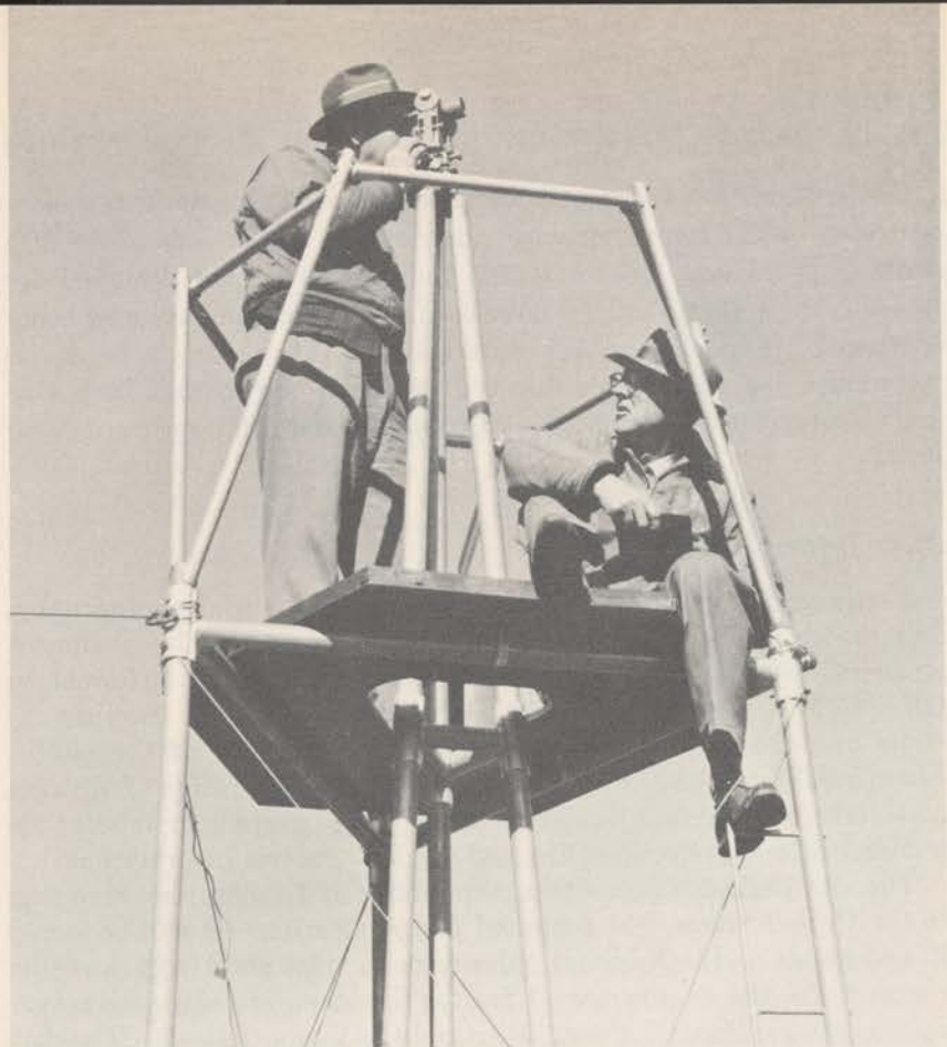
Survey topographic engineers measuring angles with a theodolite atop portable tower.
