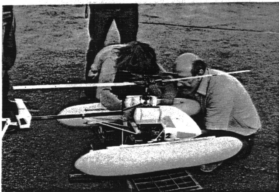
Fig. 35. A radio-controlled helicopter flown from a full-sized helicopter in flight carried an 18 kg payload at 70 km/h in temperatures below freezing.
