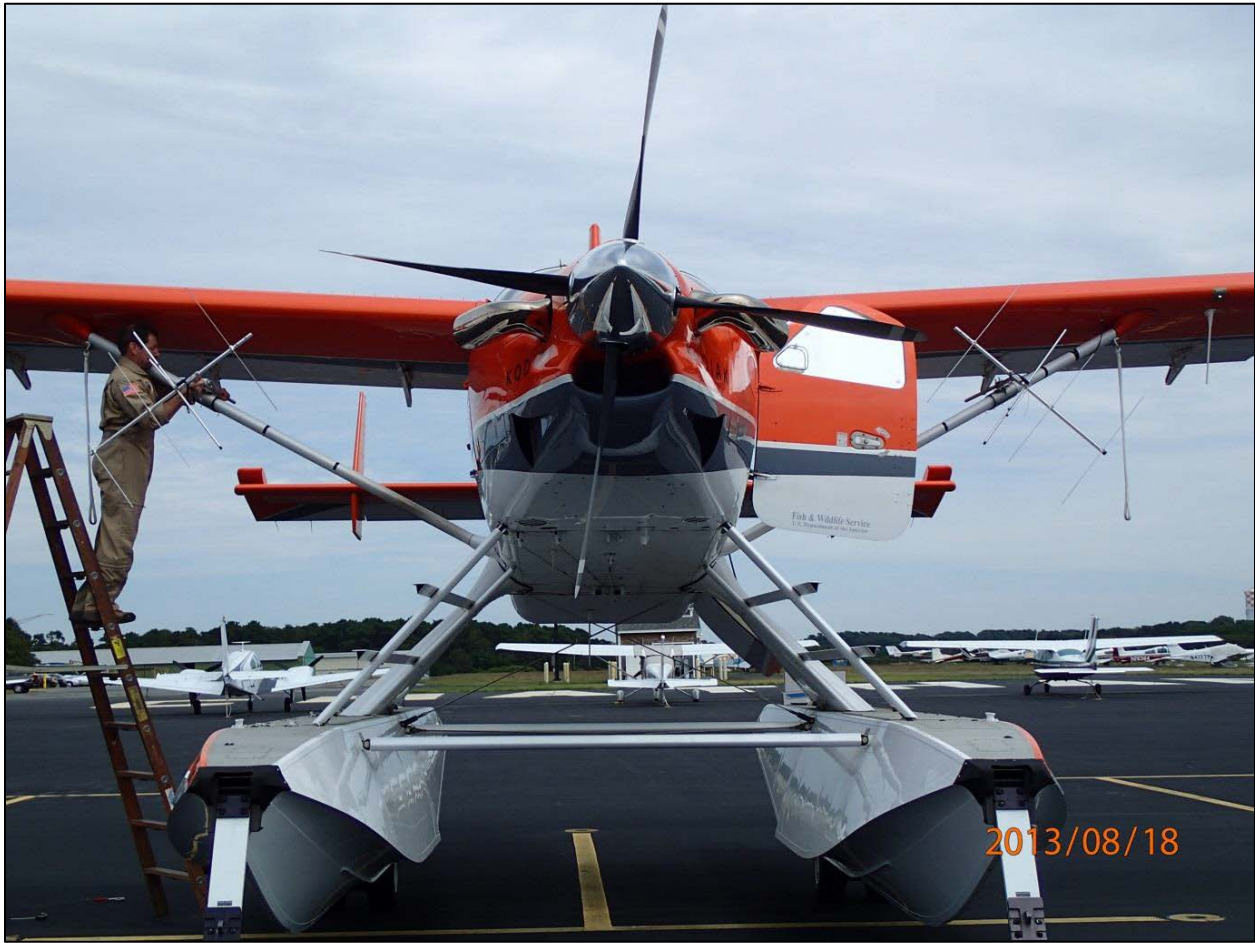
Figure 6. USFWS amphibious Kodiak aircraft with paired directional (Yagi) antennas used for aerial telemetry surveys in 2014 and 2015.
