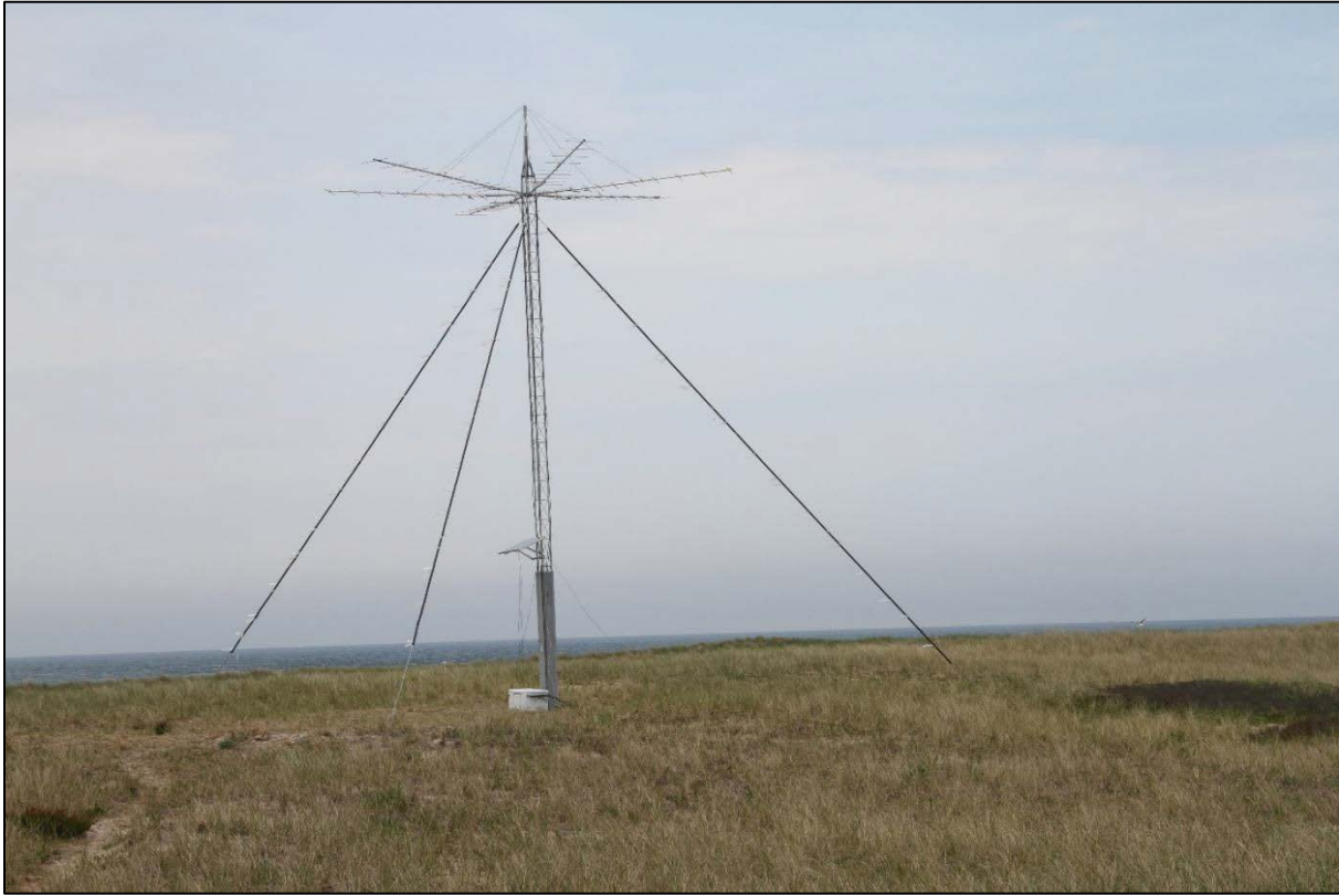
Figure 4. Automated radio telemetry station on Nantucket NWR (Great Point), Nantucket, MA Station consisted of a radial Yagi antenna array atop a guyed, 12.2 m mast with a solar powered automated receiving unit at the base (photo: Matt Malin).
