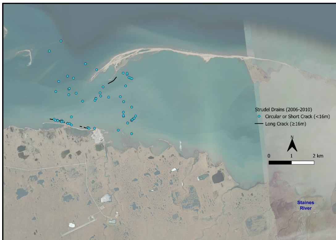
Figure 56. Strudel drains mapped near the Staines River
