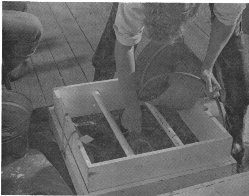
Figure 6-4. Top. Stand for elutriation of macrobenthos samples. Overflow from galvanized bucket falls down through 0.5 mm mesh screen in drawer below. Bottom. Washing the "heavy" fraction remaining after elutriation through detachable 0.5 mm mesh Nitex screen.
