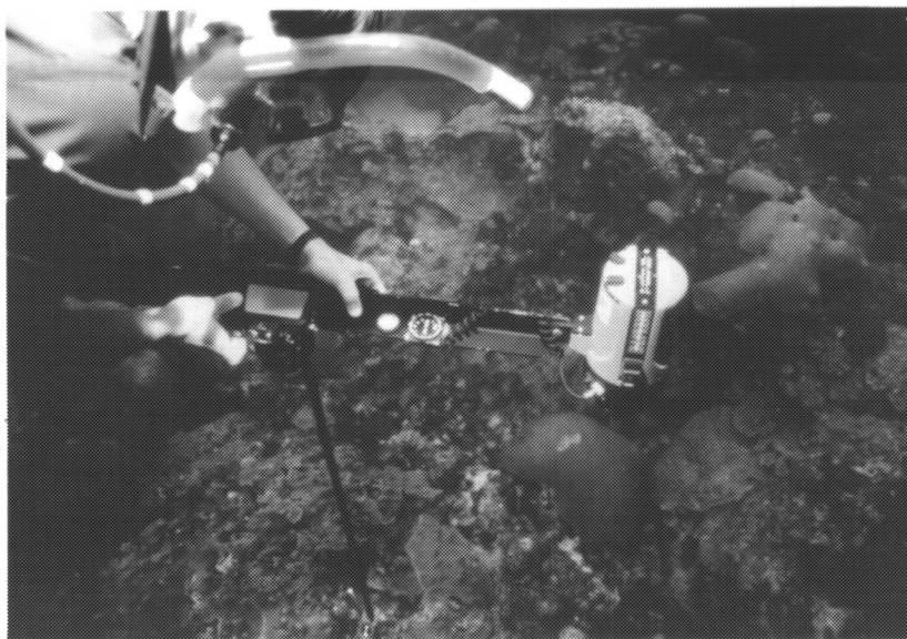
Figure 2.3. Compass and bubble level mounted on the top of the T-frame used to photograph each 8m 2 repetitive station. (These are used to adjust attitude of unit at each station prior to photography).
