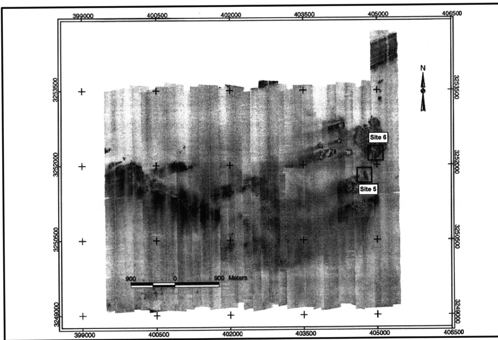
Fig. 4.13. TAMU 2 side-scan sonar mosaic of Megasite 3, showing Monitoring Sites 5 and 6 (small boxes). Conventions as in Fig. 4.10.
