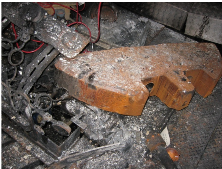
Photograph 4 - Crankshaft counterweight from DG5, A1/B1 cylinder. Counterweight was ejected from engine and landed between DG5 and DG6 in the primary burn area.
