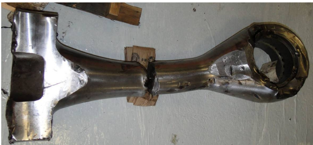
Photograph 5 - B1 Connecting Rod for DG5 Post-casualty photo provided by Wartsila
