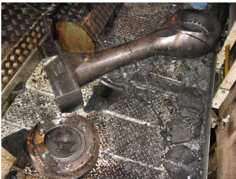
Photograph 1 - Connecting rod, upper part A1 (780 lbs) ejected from DG5 and found on deck plates in aft engine room.
