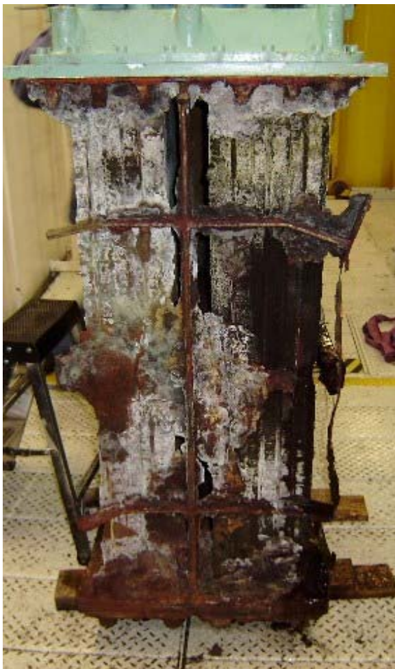
Photograph 7 - Corroded heat exchanger from DG5. Photo provided by Wartsila, taken on July 12, 2010
