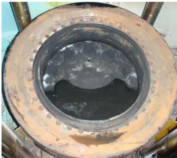
Photograph 6 - DG5, B1 cylinder liner, piston crown and gasket Photo taken by Carnival employees during head gasket replacement on November 5, 2010
