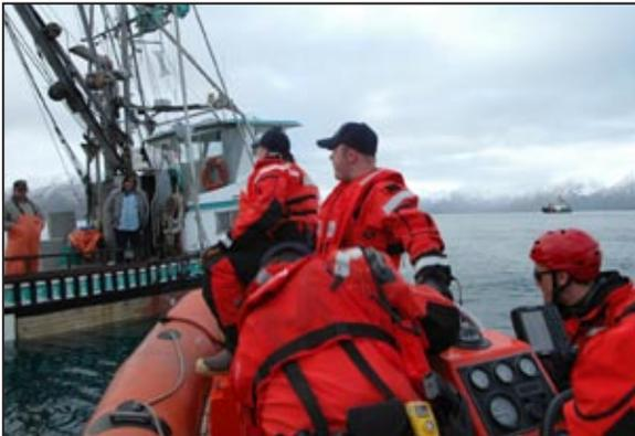
**Coast Guard boarding team members prepare to perform a safety inspection on a fishing vessel. They check the overall condition of life rings, survival suits, and other safety and lifesaving equipment onboard.**
