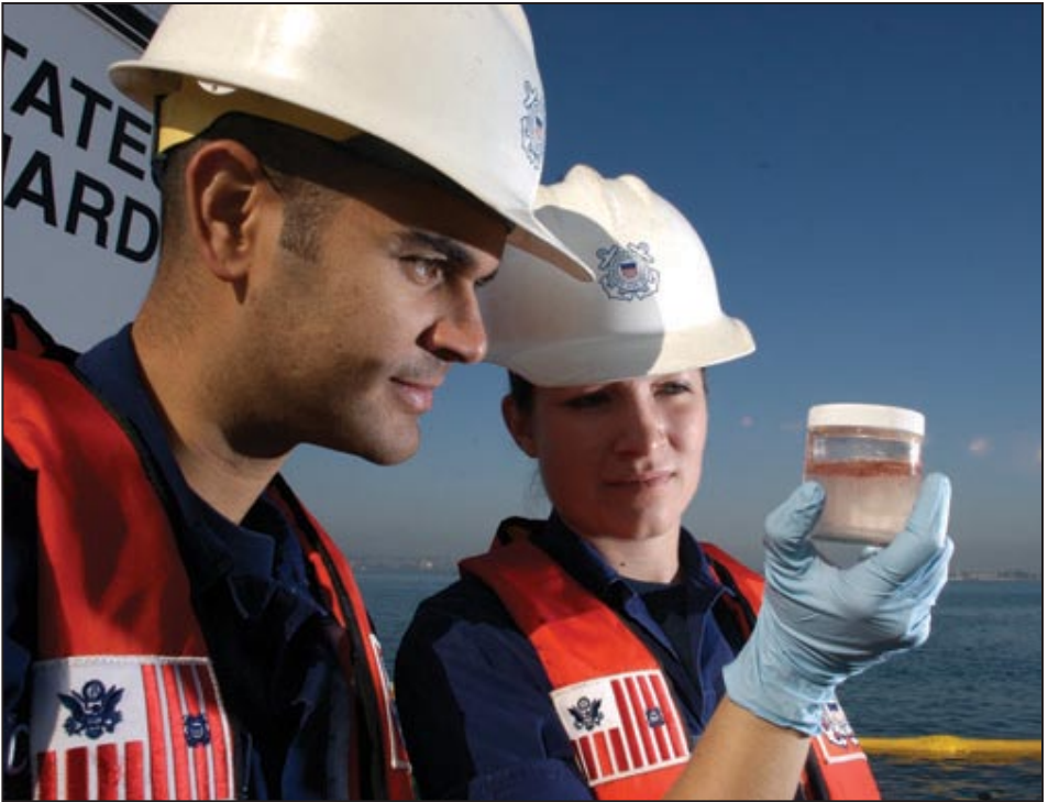
Two Coast Guard members examine a sample taken from an oil spill. Through forensic oil analysis, the USCG Marine Safety Laboratory can often determine who is responsible for the spill by comparing samples like these to oil samples from vessels in the area.
