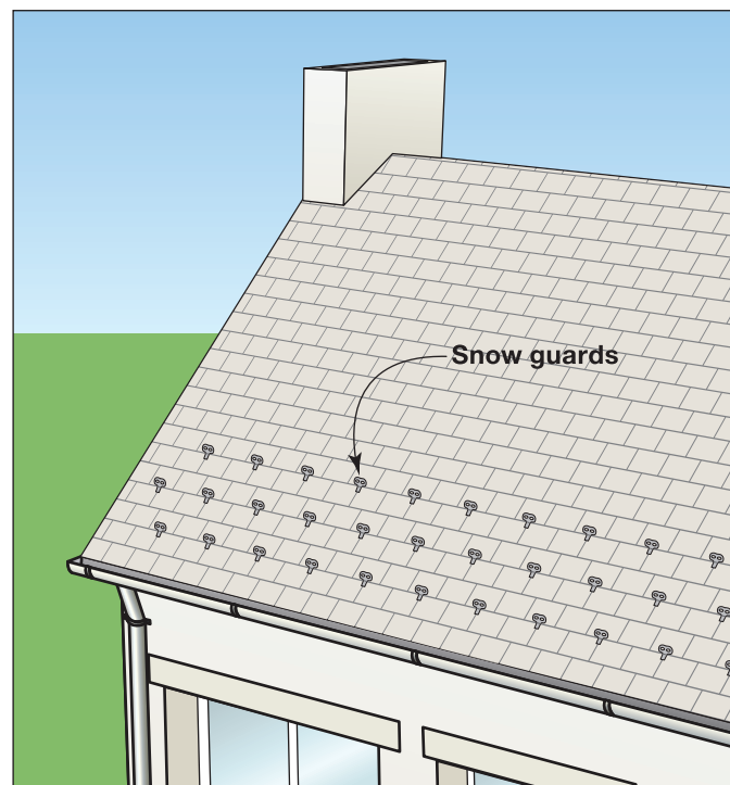
Figure 2. Snow guards or snow cleats
