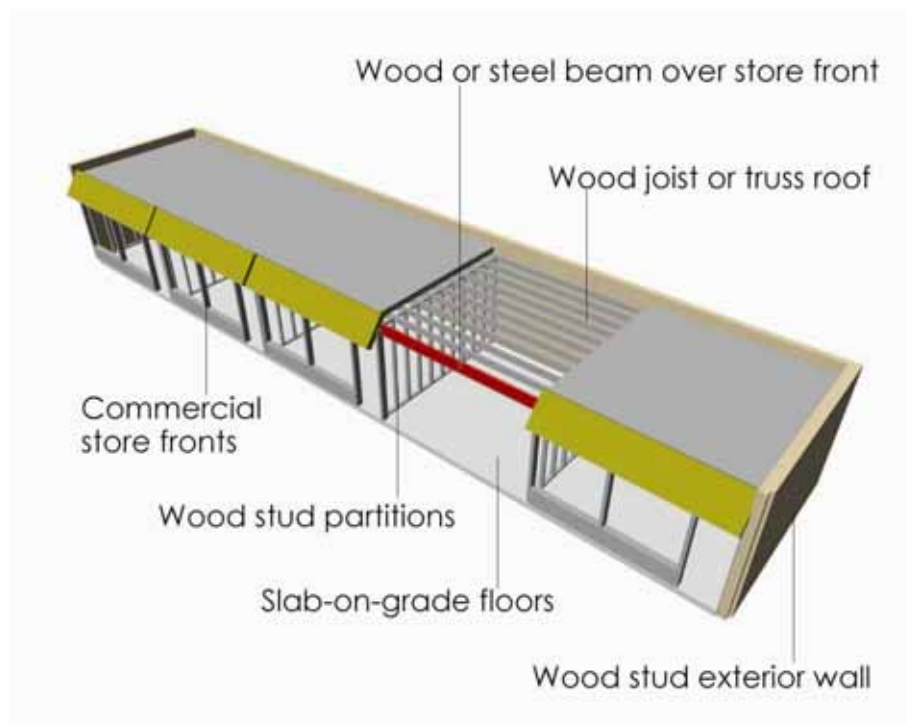
Figure 7.1-1: Building Type W2: Woodframes, Commercial and Industrial
