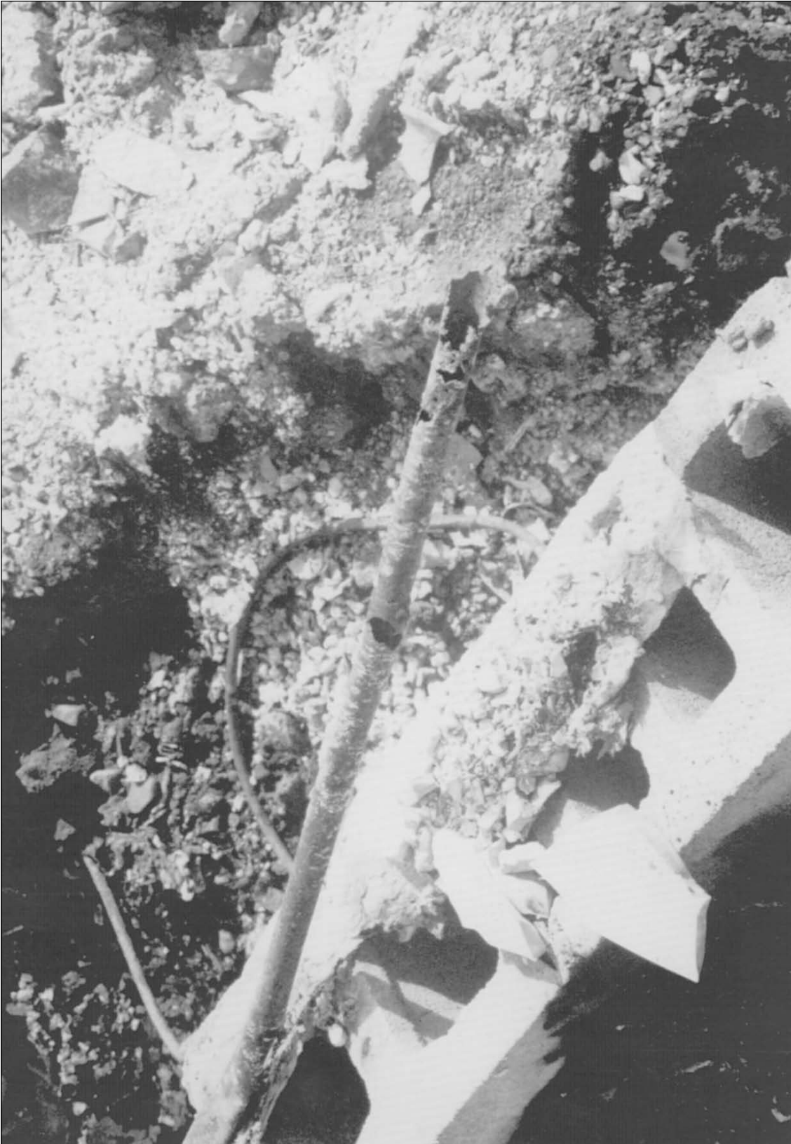
Damage to 3/4-inch copper water pipe from intense heat of the fire.
