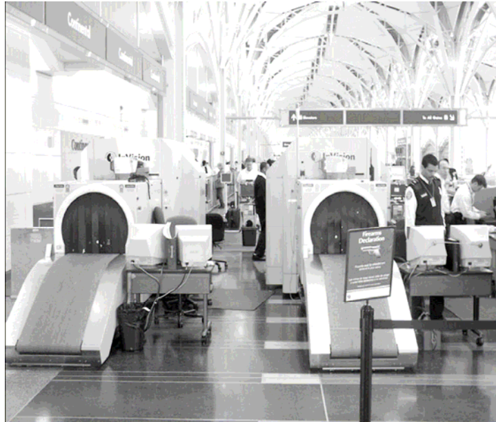
Figure 3: EDS Machines Used by TSA to Screen Checked Baggage
