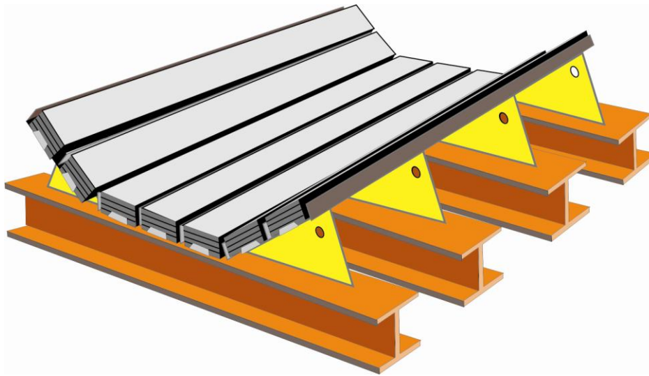
Figure 5.8. Depiction of an impact cradle with underlying rubber layers.
