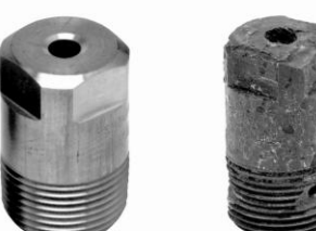
Figure 2.18. Temperature damage—new versus used [SSCO 2004].
