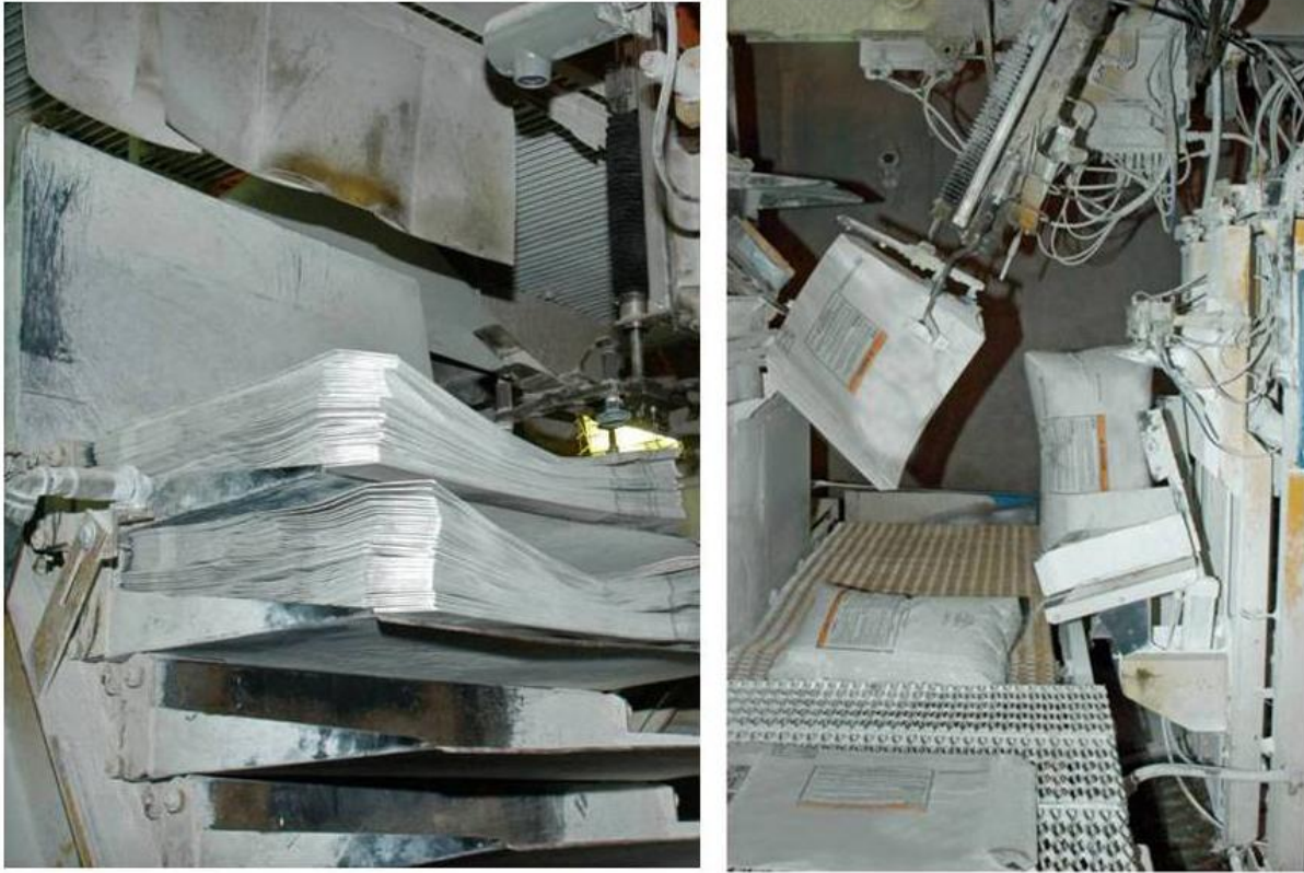
Figure 6.13. Bag storage shelves shown on left; a robotic arm with suction cups to place empty bags on fill nozzle shown on right.
