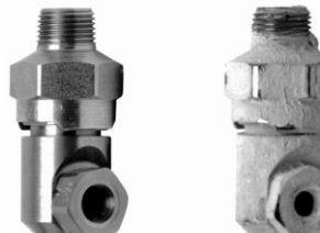
Figure 2.17. Nozzle caking—new versus used [Schick 2006].
