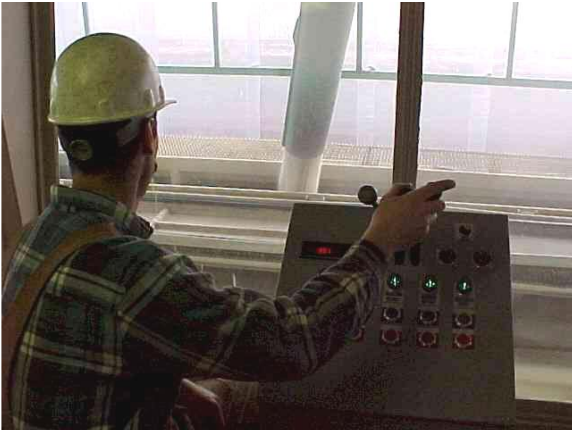
Figure 7.8. Environmentally controlled operator's booth near loadout area.
