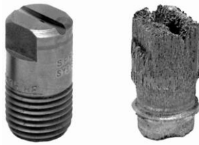
Figure 2.16. Nozzle corrosion—new versus used [Schick 2006].
