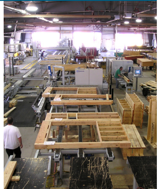
Quadrant Homes, a Building America builder in Bellevue, Washington, builds its wall panels in a factory to ensure consistency and shorten site construction time.
