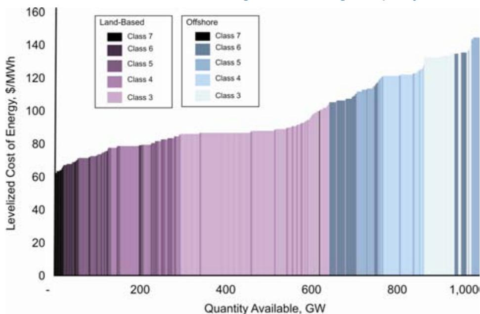
Note: See Appendix B for wind technology cost and performance projections. Excludes PTC, includes transmission costs to access existing electric transmission within 500 miles of wind resource.
