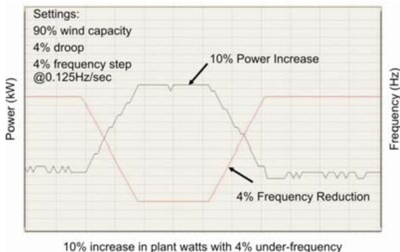
Figure 4-5. Vestas wind turbine control capability
