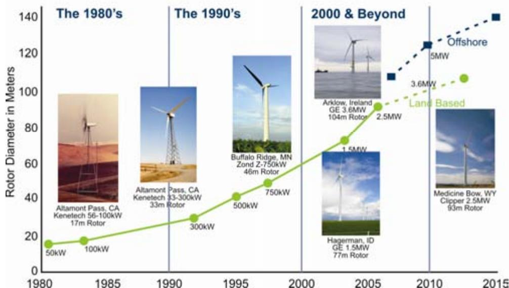
As discussed in Section 2.2.2, this long-term drive to develop larger turbines is a direct result of the desire to improve energy capture by accessing the stronger winds at higher elevations. (The increase in wind speed with elevation is referred to as wind shear.) Although the increase in turbine height is a major reason for the increase in capacity factor over time, there are economic and logistical constraints to this continued growth to larger sizes.
