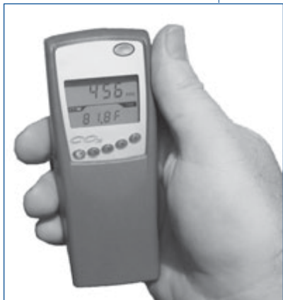
Handheld CO 2 sensor with data logging.
