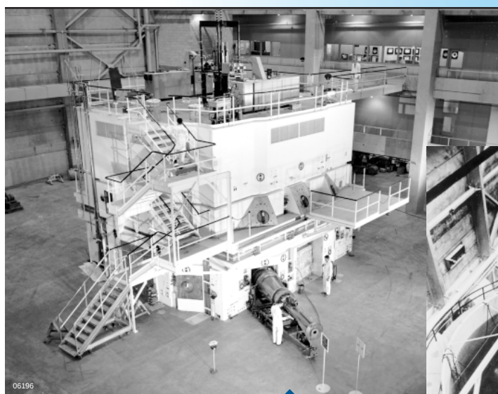
Materials Testing Reactor (No. 30) was the second reactor built at the National Reactor Testing Station, now the INL. It was used to test the performance of materials in intense radiation environments.
