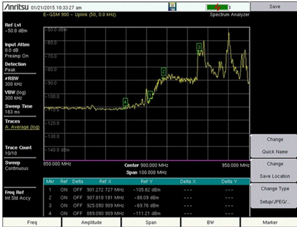
Figure 67: Example of jammer configuration problems
