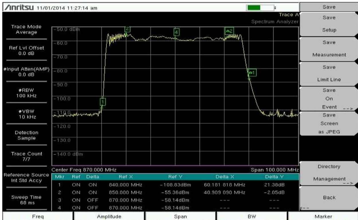
Figure 69: Output of CDMA-850 jammer from the Kabul Central Jail
