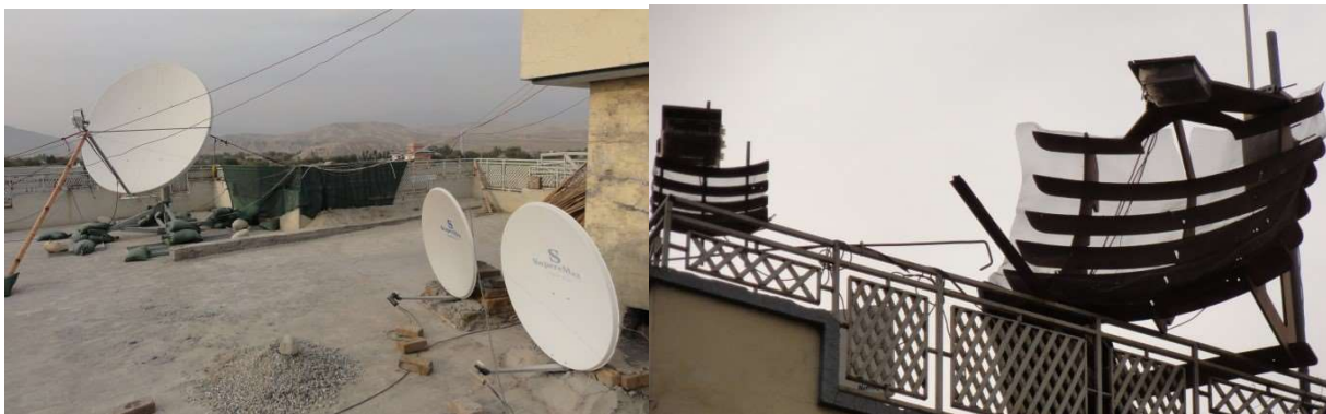
Picture 34: FabFi RF reflectors and satellite dishes on the roof of the Taj
