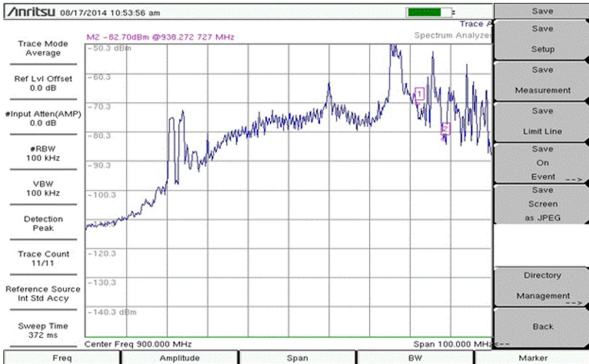
Figure 66: Uplink jamming example for the GSM-900 band
