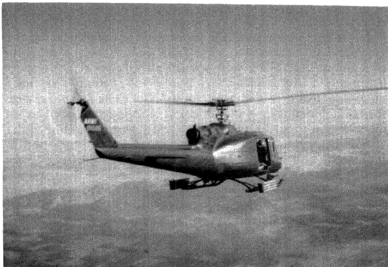
Early in the war, a Huey gunship (above) carrying two mini-guns and rockets flies support cover. Beginning in 1967, the AH-1G Cobra (below) replaced the Huey in its gunship role.
